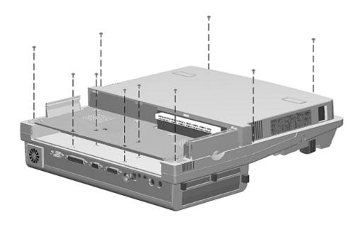
Figure 7-11. Removing the Bottom Cover Screws
